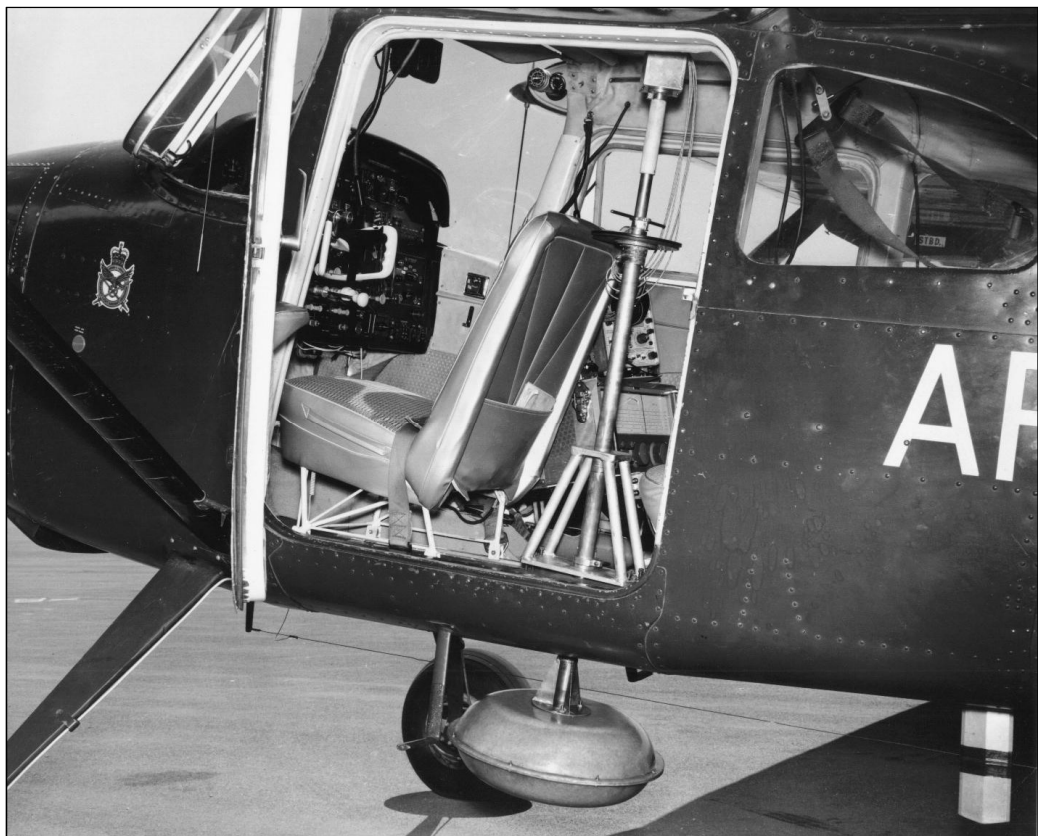
Photo 5-1.7 - Cessna 180A fitted with ARDF equipment.
