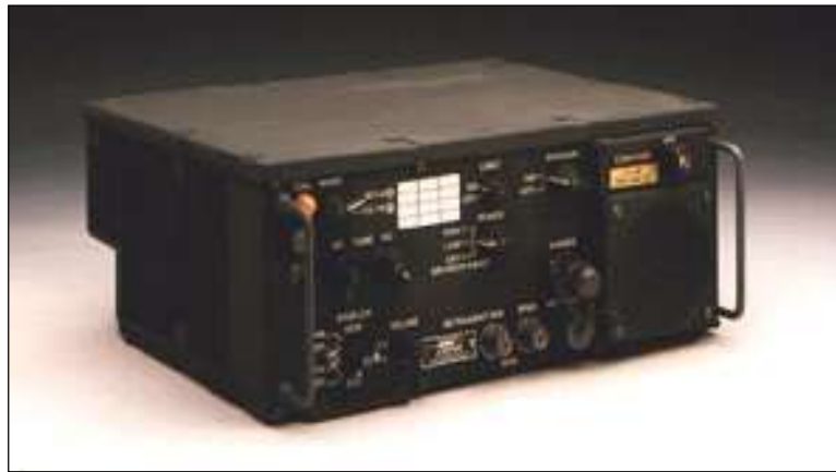
Photo 1.5 - RT-524 Transceiver (Part of AN/VRC-12 series).
