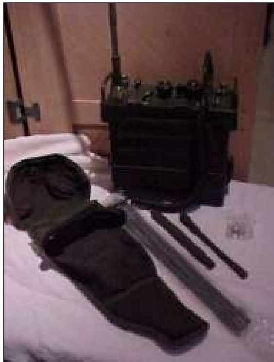
Photo 1.3 - AN/PRC-25 VHF Radio Set with two antennas and accessory bag.
