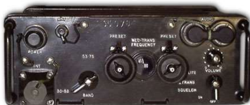
Photo 1.4 - AN/PRC-25 VHF Radio Set - Front panel layout.
